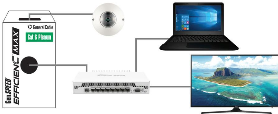
\* 0.6A is the ampacity rating of the cable, which equates to 120 watts using 50 volts over four pairs.
