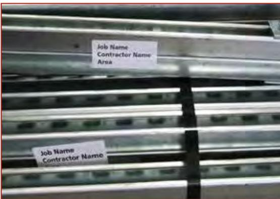
*Trapezes and Assemblies can be labeled to correspond with specific locations on drawings.*
