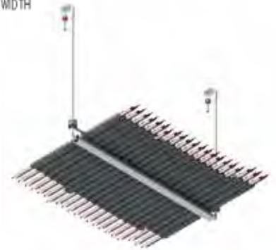
Tip..."Rollers" can be added to the crossbar to help the MC slide through the supports. Just ask!
