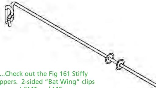
Tip...Check out the Fig 161 Stiffy Grippers. 2-sided "Bat Wing" clips to support EMT and MC.
